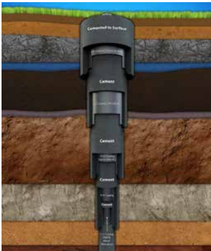
Exhibit 4-9. Components of the well construction process
